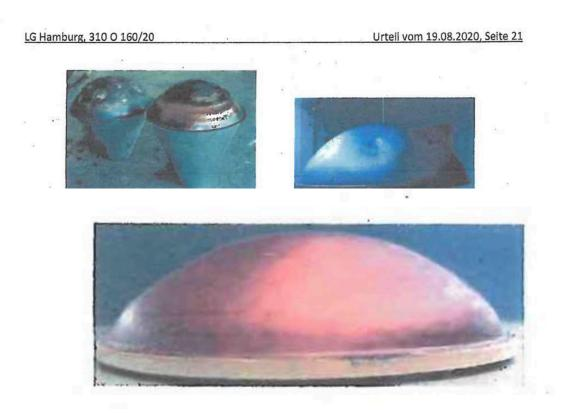
These pictured proposed shapes stand by far the strongest of all in Panart's argumentation. The functionality of the pan face on the top shell is not severely compromised by these ways of clamping the top shell, as long as they still allow the whole resonance body to act similar to a Helmholtz resonator.
